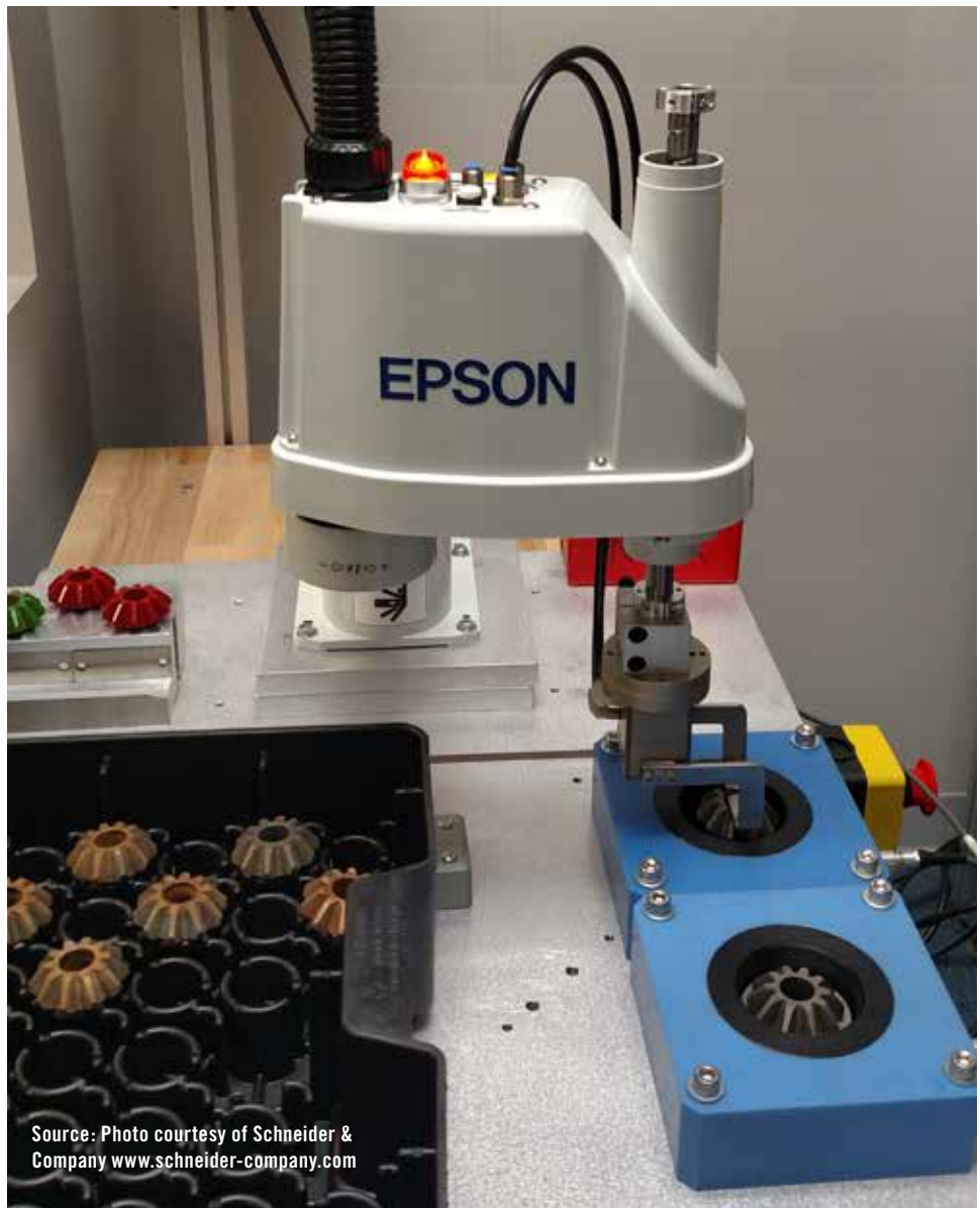
Figure 3: Epson robot and demo gear-test station: The robot is programmed to pick up a part from the parts tray on the left and place it into the eddy current coil closest to the robot. Three colored gears on the left side of the photo are test standards used to validate the testing process.
