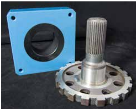
Figure 1: Complex gear and eddy current probe
